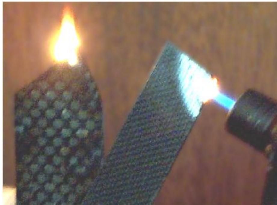
**A carbon-epoxy composite (left) is burning while a Carbon-Geopolymer Composite still resists a 1200 deg.C fire**
