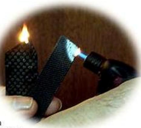
A carbon-epoxy composite (left) is burning while a Carbon-Géopolymère Composite™ still resists a 1200°C fire
