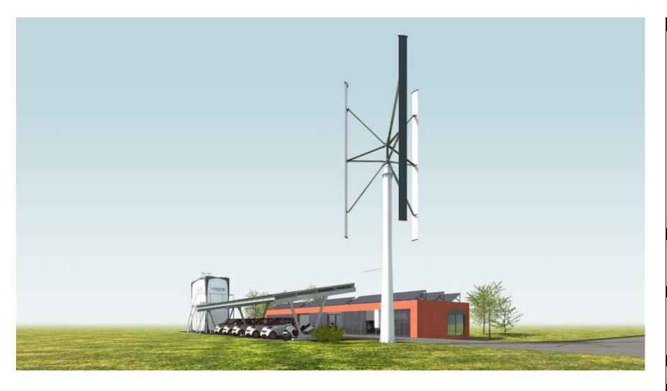
The station uses different renewable sources to ensure operation of a fleet of electro-cars, electro-scooters, electro-bikes and other technologies. It works in off-grid or semi off-grid mode.
